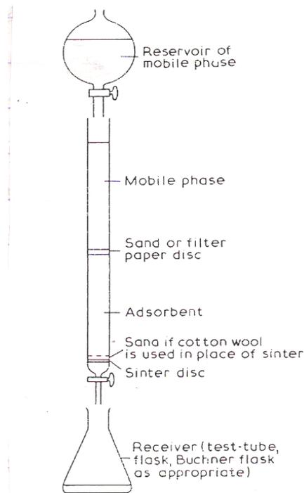
Fig.8- Apparatus for column chromatography.
