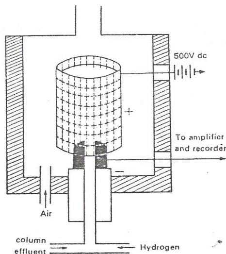
Fig.9- Hydrogen flame ionisation detector.
