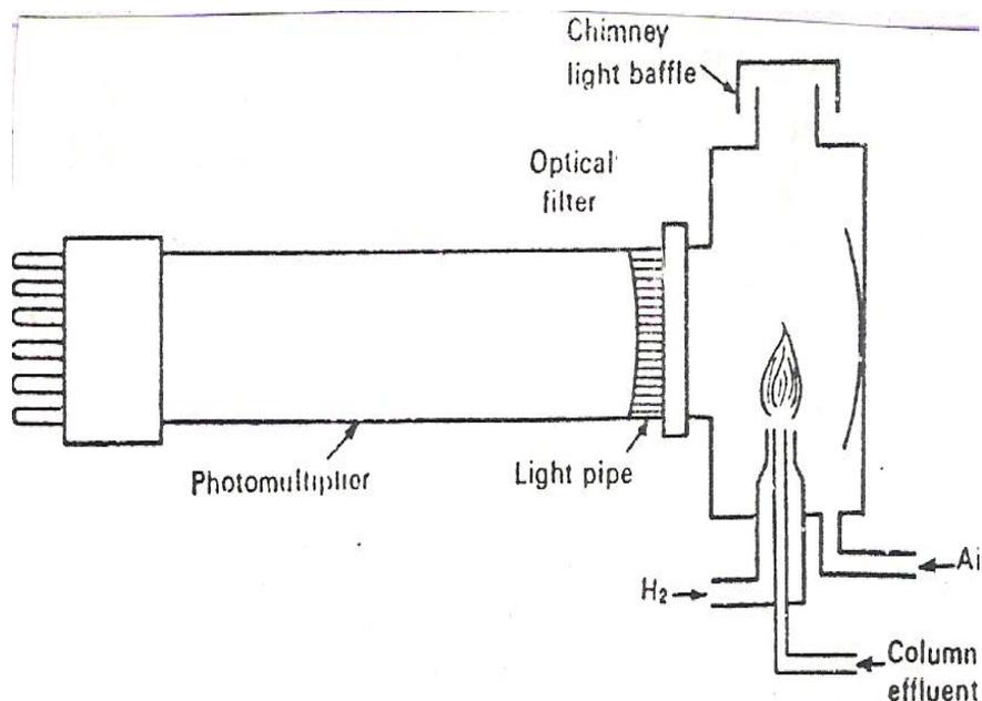
Fig.10- Flame photometric detector.
