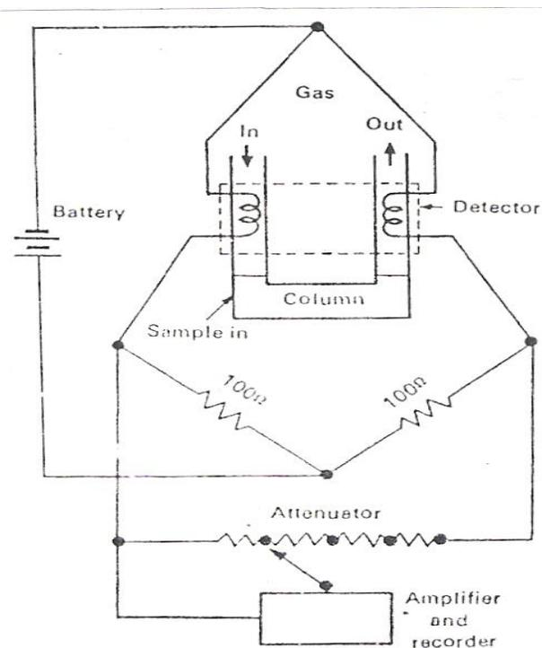
Fig.11 – Thermal conductivity detector.
