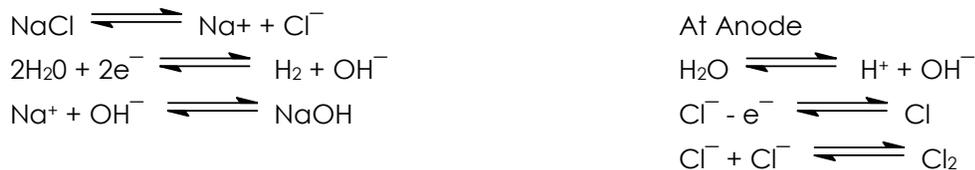
Since chlorine attack caustic soda solution even in the cold, formed sodium chloride and hypochlorite, it is necessary that the construction of the cell should be such that NaOH and Cl<sup>-</sup> once formed do not come in direct contact with one another.
