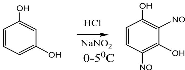
**PROCESS:** Dissolve 10gm resorcinol in 100ml of water. Add 20cc HCl and 25gm NaCl in above solution. Add ice and bring temperature to 0°C. Stir the solution mechanically. Prepare a solution of 13gm sodium nitrite in 50ml water. Allow nitrate solution to flow very slowly. This takes about 60 minutes. When liquid show acidic nature, allow stand for one hour. Filter the precipitate, wash with cold water and dry.
