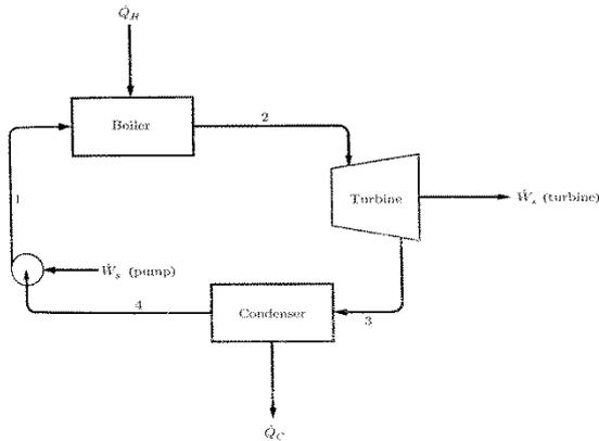
Figure 1: Simple steam power plant.
