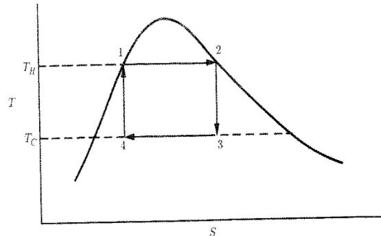
Figure 2: Carnot cycle on a TS diagram.
