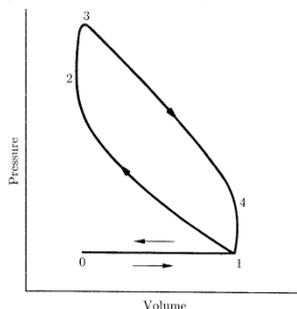
**Figure 5:** Otto internal combustion – engine cycle
