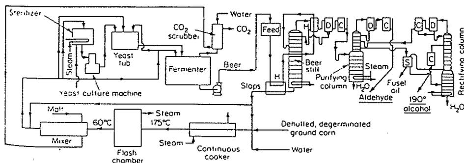
Flowsheet for industrial alcohol. KEY: C, condenser; D, dephlegmator; H, heat exchanger; S, separator
