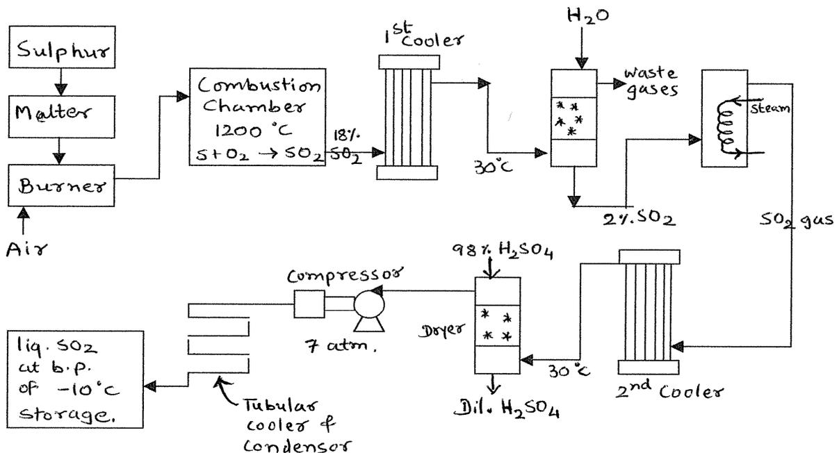
Then the 18% SO<sub>2</sub> from combustion chamber is sent to the 1<sup>st</sup> cooler where it is cooled at 30°C. Then it is passed through **absorber** from top of which water is percolated. Here SO<sub>2</sub>
